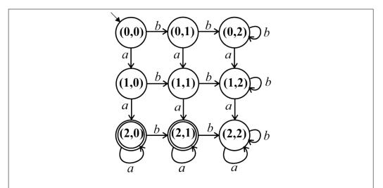
**Figure 5.6.** A DFA recognizing strings of a's and b's with at least two a's and at most one b.
