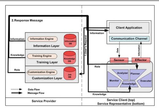
Fig. 4 Proposed architecture. Based on the client's request, the service provider generates a 3-segment response message to customize and train a client-side generic agent as its representative to serve the client
