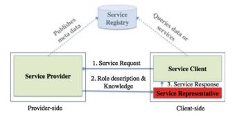
**Fig. 1** Proposed extended SOA model. The *shaded area* represents the non-essential component (service registry) in the SOA model. This model also supports the traditional service invocation where the service provider returns the service response directly to the service client
