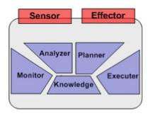
**Fig. 3** Structure of an autonomous software agent, called MAPE-K (monitor-analyze-plan-execute over a knowledge base), proposed by IBM [22]
