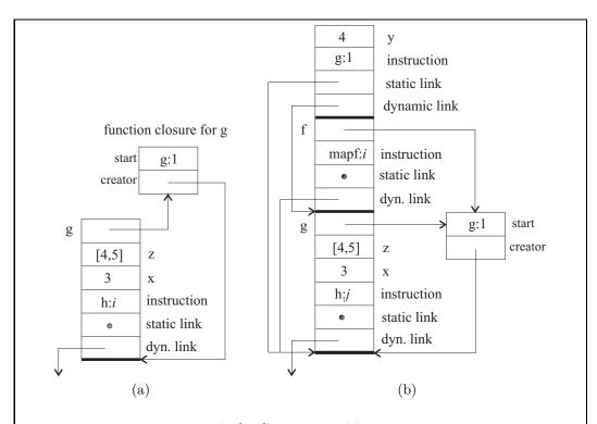
Figure 8.5: Evaluation of h(3, [4, 5]). Diagram (a) shows the frame for h in the runtime stack just before h calls mapf. Notice that the value of g in that frame is a pointer to a function closure. Diagram (b) shows the stack after h has called mapf and mapf has called g. The frame for mapf is abbreviated, showing only the value of f. Mapf gets the static link to use for g from the closure that represents g.
