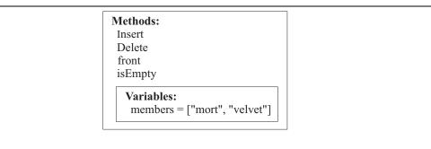
Figure 19.1: A snapshot of a queue object. The methods (Insert, Delete, front and isEmpty) are visible to other objects, but variable 'members' is private, so is only visible to the methods inside this object.
